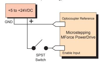
Figure 2.4.6: Switch Interface Example
